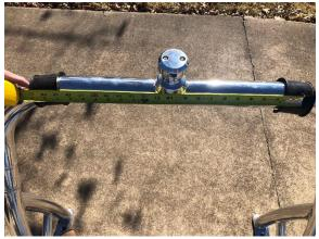
• Place The Matt Rack<sup>©</sup> onto the tow bar with the rubber adapters installed, see photo.
