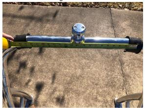
Place The Matt Rack© onto the tow bar with the rubber adapters installed, see photo.
